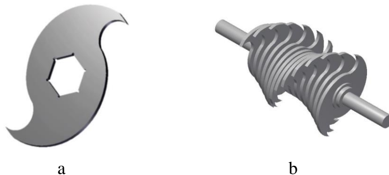
Fig. 6. Blade with two teeth (a) and shredder rotor composed of such blades (b) [8]
