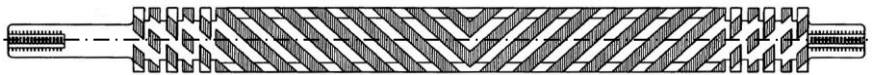
Fig. 16. Scheme of a rotor with combined cutting elements (Patent Application No. US2006/086855A1)
